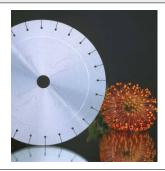
the TECHNO - Core is a solid steel core. Over the core surface laser slots are arranged. Due to this design the vibration of core and the noise level during the sawing prozess is minimised.
