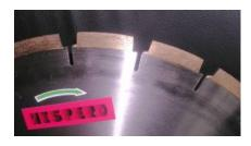
the WISPERO - or Sandwich-Core has on the outside each a hardened and grinded Steel layer with inside a copper layer. By this special sandwich design the vibration of core will be minimised. Due to this effect the noise level during the sawing prozess is minimised.
